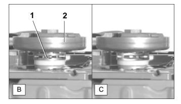
Check the sprocket (B/1) before mounting a new chain. The sprocket is located underneath the clutch drum (B/2).
